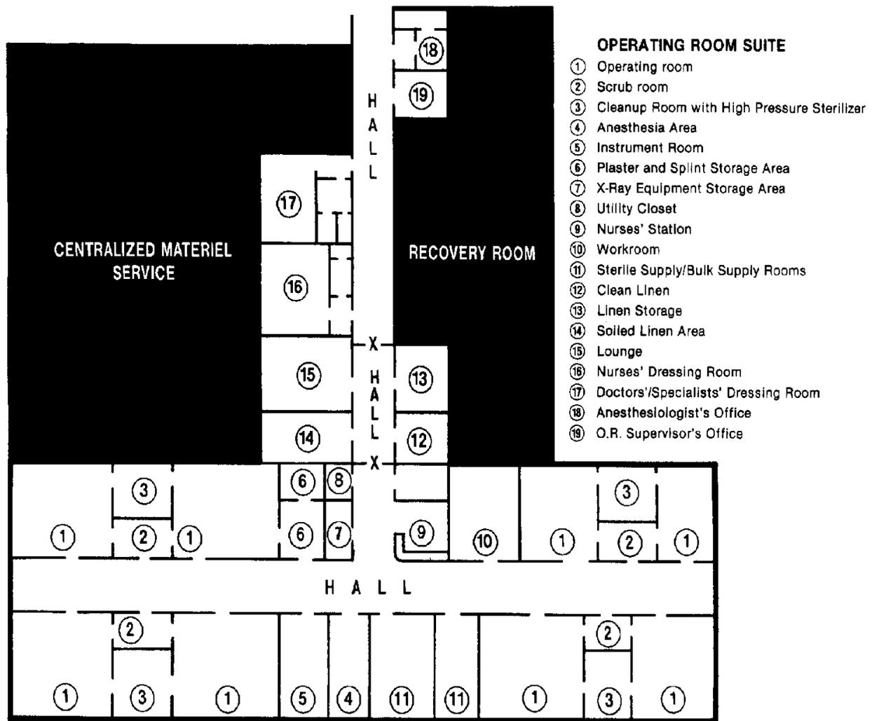
Figure 1-3. Type floor plan for an Army hospital operating suite.
