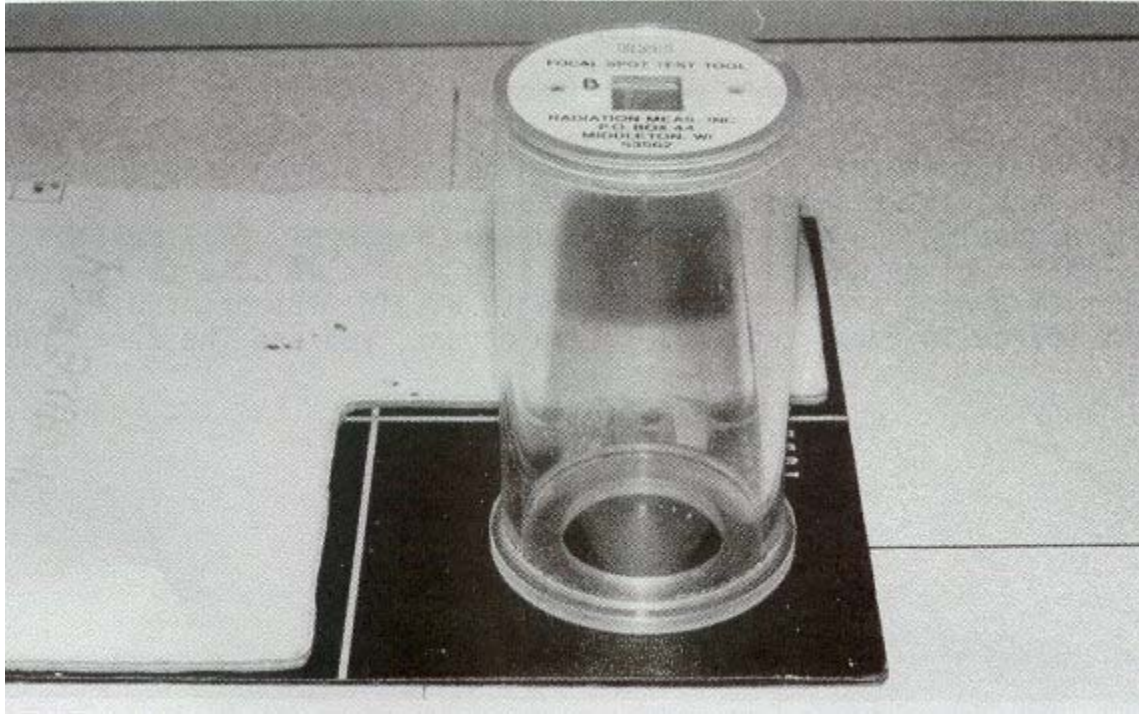
Figure 4-13. Both exposures of test tool using large focal spots. Note "B" marker is used for large focal spot test.
