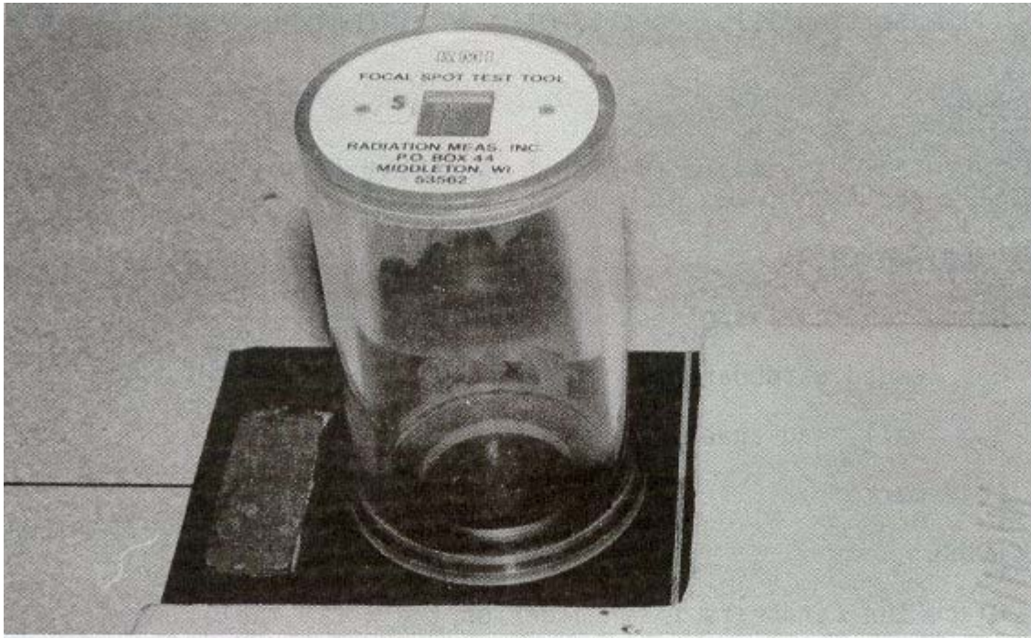
Figure 4-11. First exposure with small focal spot. Note "S" marker on top of test tool.
