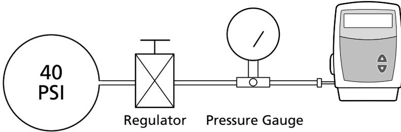
4. Connect the Medication Cassette™ Reservoir outlet tube to the metered pressure source.
