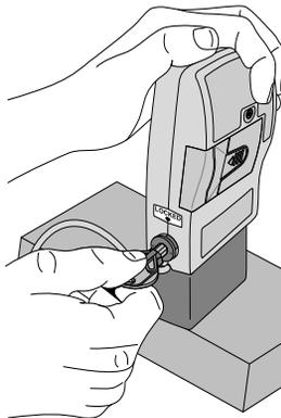
4. Insert the key into the lock, push in, and turn counterclockwise until the line on the lock lines up with the arrow on the side of the pump and you feel the lock click into place.
