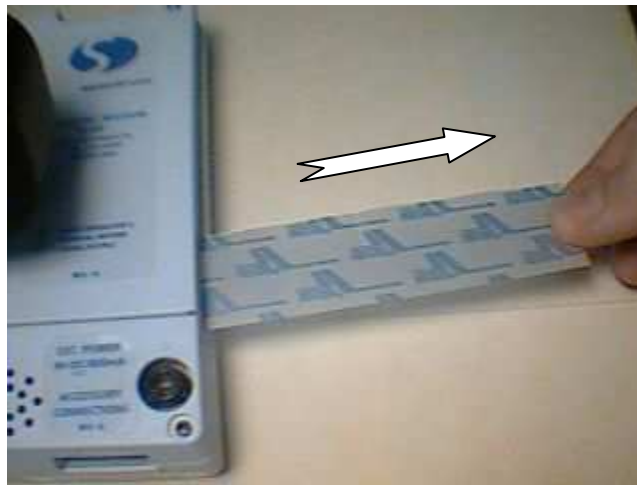
Pull the battery tab straight out from the Battery Pack cavity.
