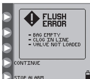
Figure 29. Flush Error screen.
