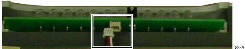
6. Remove the defective alarm light PCB and set aside.
