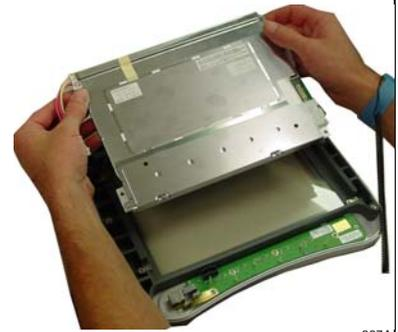
3. Dampen a clean, soft cloth with window cleaner and carefully clean and dry the new LCD display and the display filter to remove fingerprints and dust particles.
