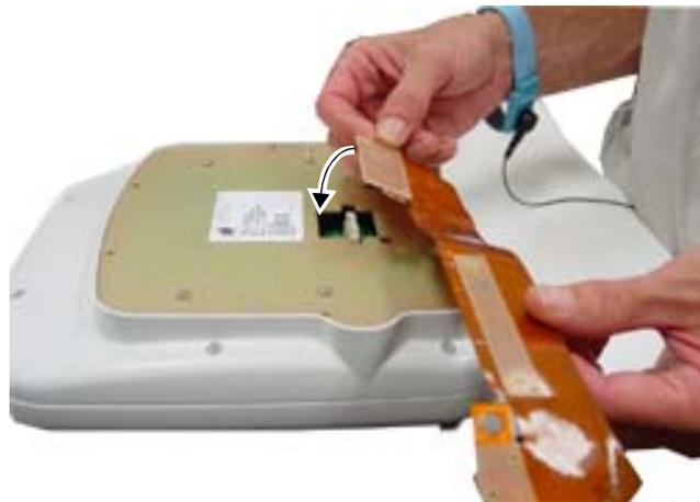
5. Using two flathead screws from the kit, secure the flex cable to the display assembly.
