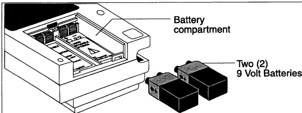
**CAUTION:** To assure proper pump operation, always replace both batteries with fresh alkaline batteries when a change is required.
