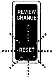
Press [RESET] before pressing [ENTER] to return an incorrect numeric value to zero.
